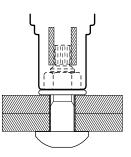
Slide the inner socket over the bolt tip and the outer socket over the nut. Press the trigger switch. The outer socket will rotate and tighten the nut until the bolt reaches the required tension.
